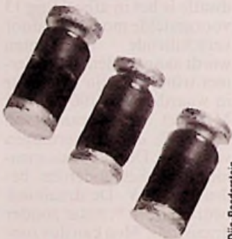
Afb. 20 Dioden in SOD-80 omhulling.
